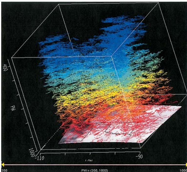
**FIG. 13.** VisAD display [latitude–longitude–altitude (hPa) cube] of simulated GIFTS winds illustrates the data density and vertical distribution that could be achievable from hyperspectral sounders of the future.
