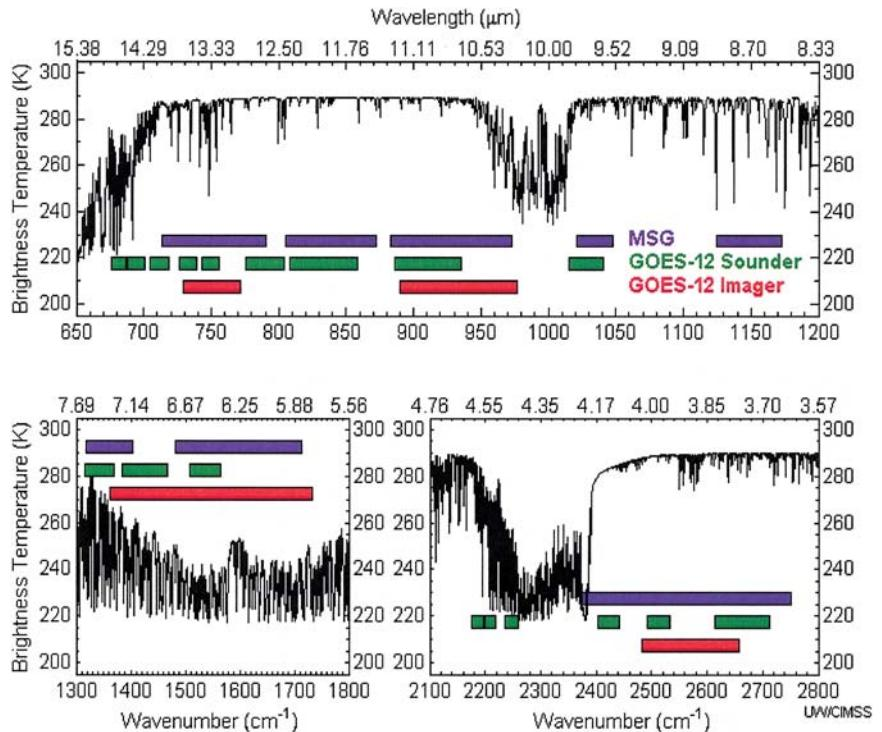
**FIG. 12.** A segment of the electromagnetic spectrum as observed at the top of the atmosphere together with the infrared spectral band coverage of the MSG SEVIRI instrument. For comparison, the spectral coverage of the GOES-12 sounder/imager is also shown.
