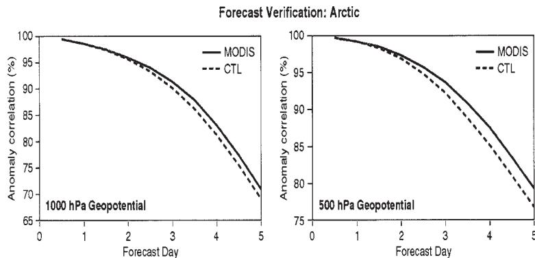
**FIG. 9.** Anomaly correlation as a function of forecast range for the (left) 1000- and (right) 500-hPa geopotential height forecast in the Arctic region (north of 65° latitude) from the ECMWF MODIS winds impact experiments. The MODIS experiment (solid) and the control experiment (dashed) have each been verified against their own analyses. The study period is 5–29 Mar 2001. (From: Key et al. 2003.)
