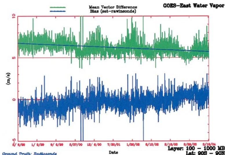
**FIG. 11.** Mean vector difference (green) and speed bias (blue, satellite – rawinsonde) for GOES-8/-12 upper-level (100–400 hPa) water vapor winds for the period 6 May 1998–18 Mar 2004 (GOES-12 statistics began in Apr 2003).
