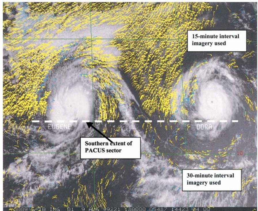
**FIG. 4.** GOES-10 low-level cloud-drift winds (yellow: 800–950 hPa, cyan: 700–800 hPa) around Hurricanes Dora and Eugene using 15- and 30-min-interval visible imagery.
